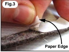
Press the raised adhesive strip back down on to the felt seal.
